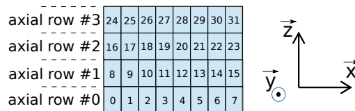
Figure 9: Pixel indexation in a SPECT gamma camera with 4 axial rows of 8 transaxial pixels.
